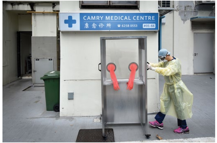
Feedback from doctors helped the team to design a booth that is lightweight and easy to wheel around.
